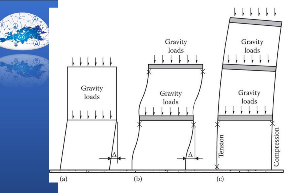
**Collapse patterns:** (a) inadequate shear strength, (b) inadequate **beam/colum**n strength, and (c) tension compression failure due to **overturning**.
