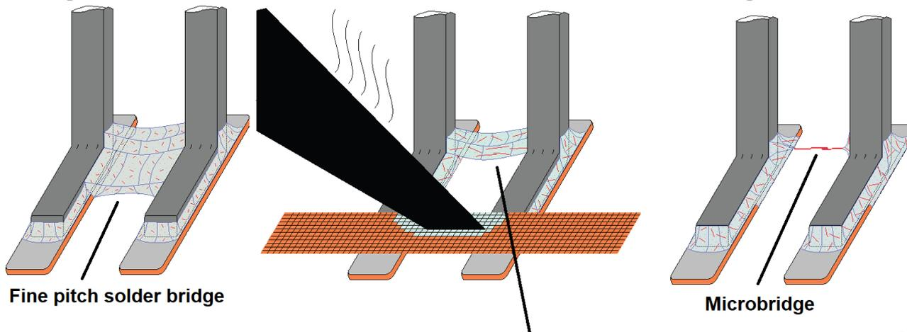
The solder saturated with copper and some  $Cu_6Sn_5$  crystals.
