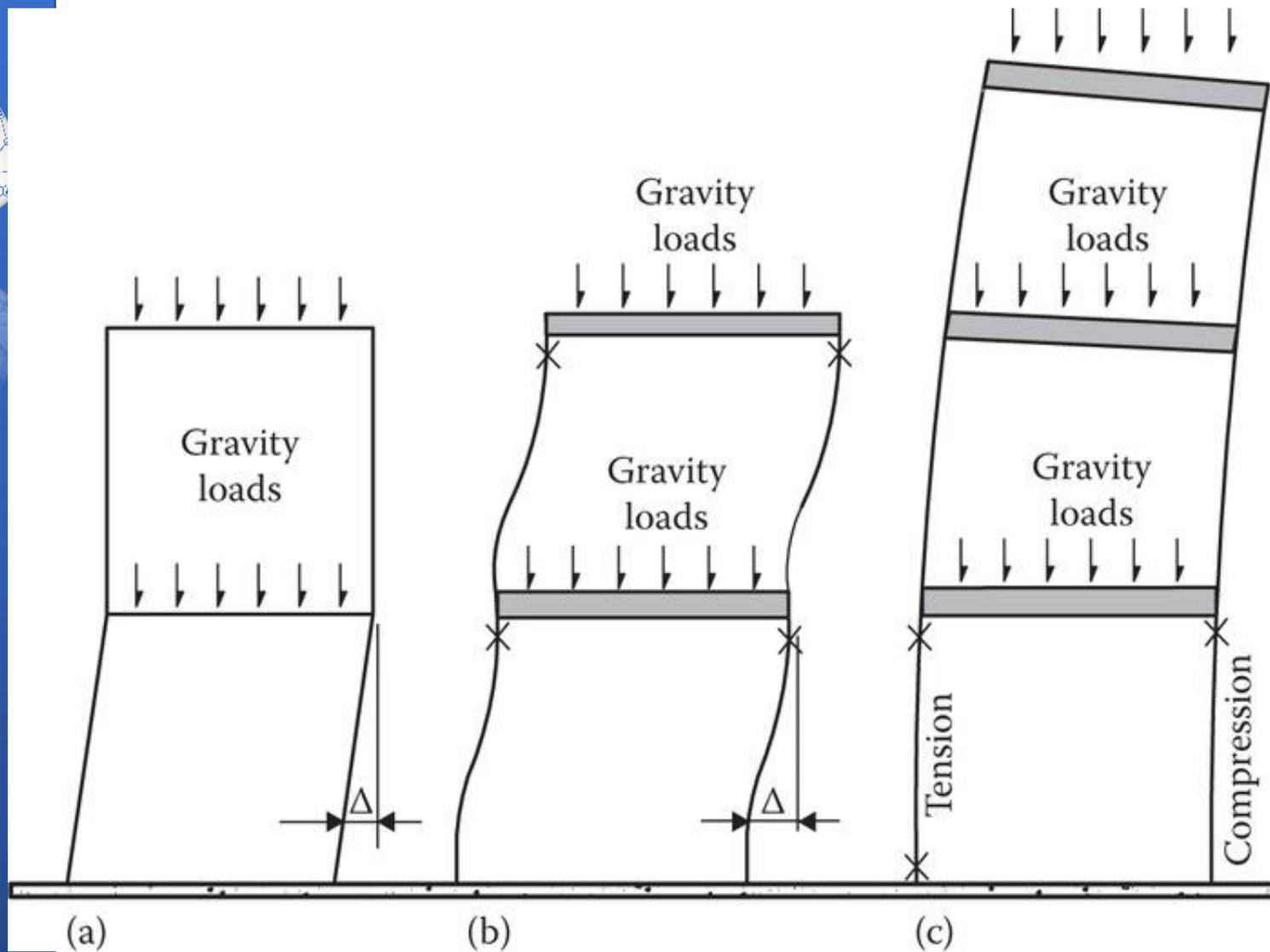
**Collapse patterns: (a) inadequate shear strength, (b) inadequate beam/column strength, and (c) tension/compression failure due to overturning.**
